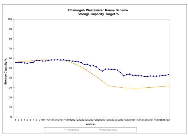
FIGURE 20. Winter Storage Dam Actual and Target Capacity
